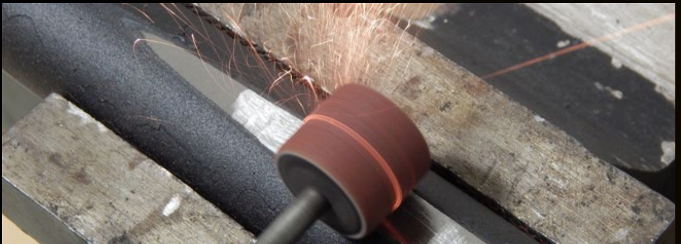
Grinding – preparation for hardness testing
