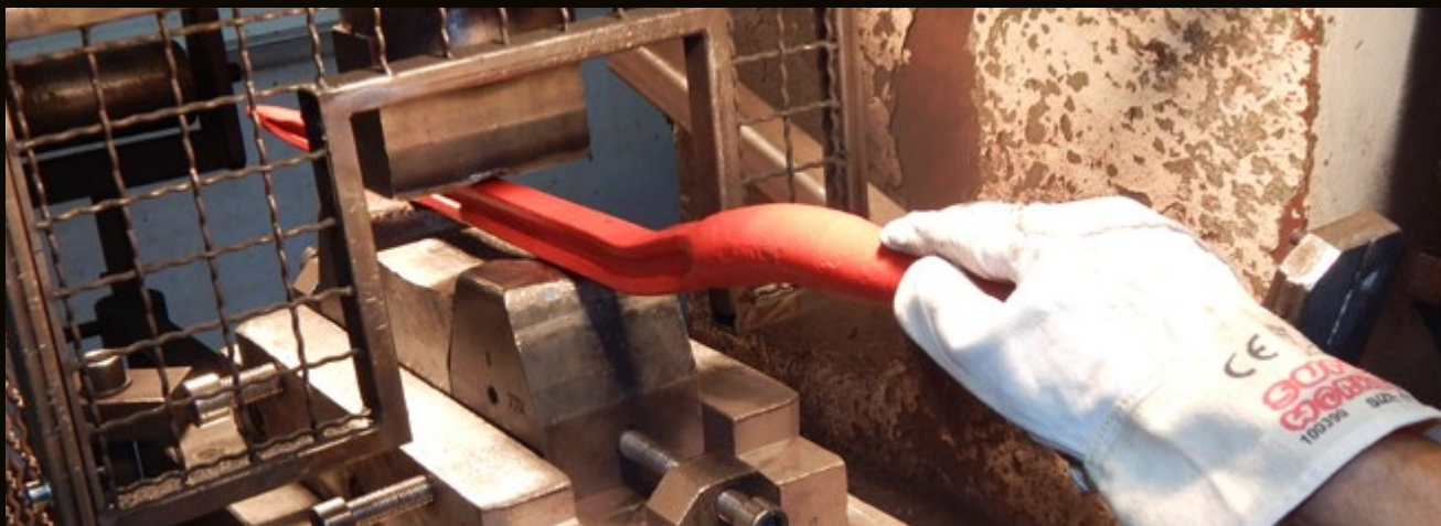
Each tine is straightened and is therefore subject to 100 % quality control
