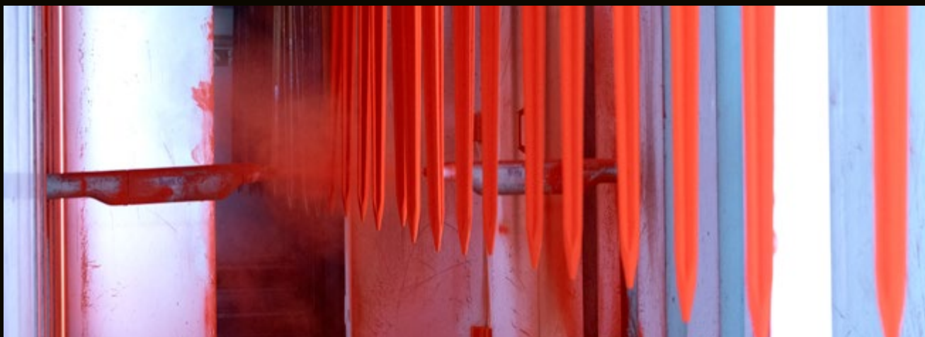
In our in-house coating facility, our loader tines are powder-coated in an environmentally friendly, solvent-free process
